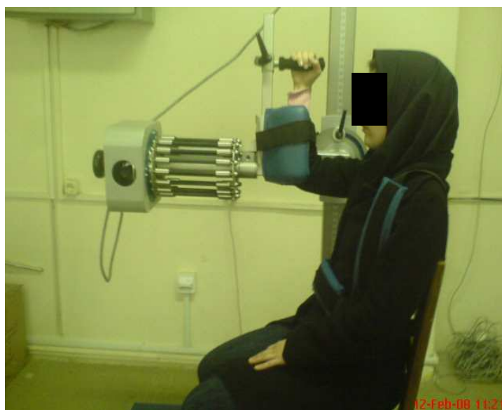
Figure 1. Measurement of maximal isometric external rotation torque
