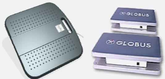
Picture 1. Picture show Libra and Twin Plates instruments
